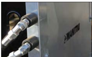
(1) Fully enclosed hydraulic components & connector sockets
